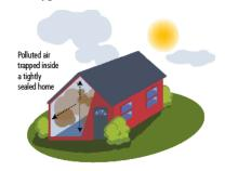
By making buildings too tight, we are locking in all of the pollutants generated inside the house (CO<sub>2</sub>, CO, smoke, odors, germs, VOCs, etc.). Those chemicals, if not dealt carefully with an intelligent ventilation system, could make the premises very uncomfortable for the residents. Furthermore, people and pets could become drowsy, get sick more frequently, and have potentially fatal consequences in extreme cases.
